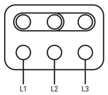
If the motor has 6 types from the winding, a star bridge (W2-U2-V2) is mounted on the terminal board.
