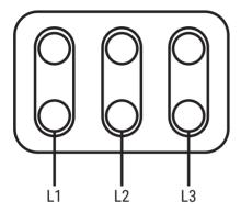
Motors for delta connection generally have 6 winding types.
